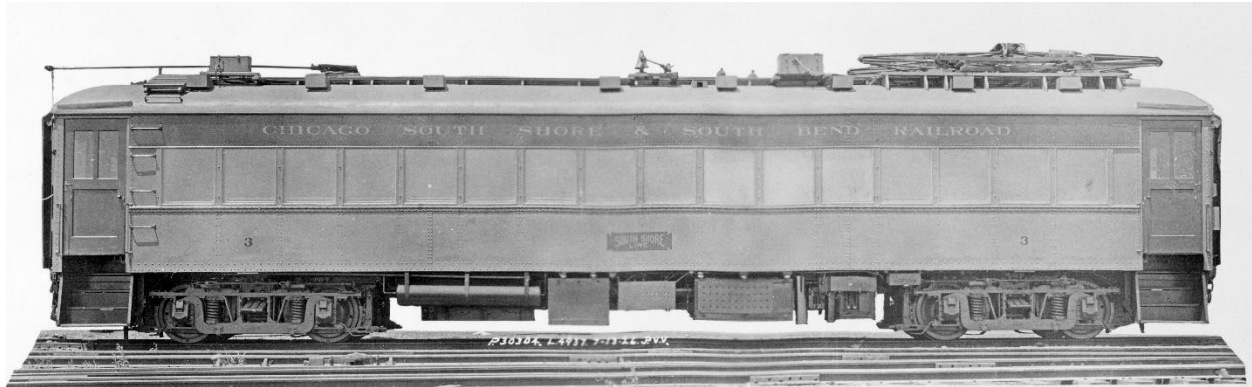
Car #3 at Pullman, 13 July 1926. The original arrangement of one pantagraph and one trolley pole was short-lived as trolley pole operation was incompatible with the double-contact trolley wire on the Illinois Central. The roof mounted bells did not last long either, perhaps a year.
