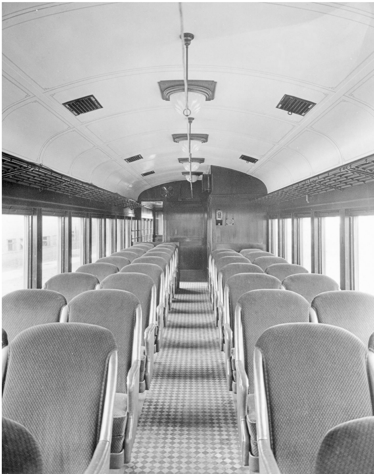
Car #27 at Standard Steel Car Co., Hammond, Indiana, January 1929. This was the most common car type on the South Shore Line, a box smoker with bucket seats – 38 of the 68 steel cars were so equipped, including car #31.
