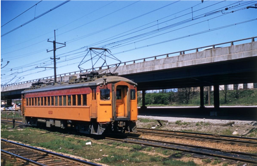
Car #4, Gary, Indiana, in the 1950s. The destination sign and train number boxes have been removed, and the plate glass end windows have been replaced with safety glass.
