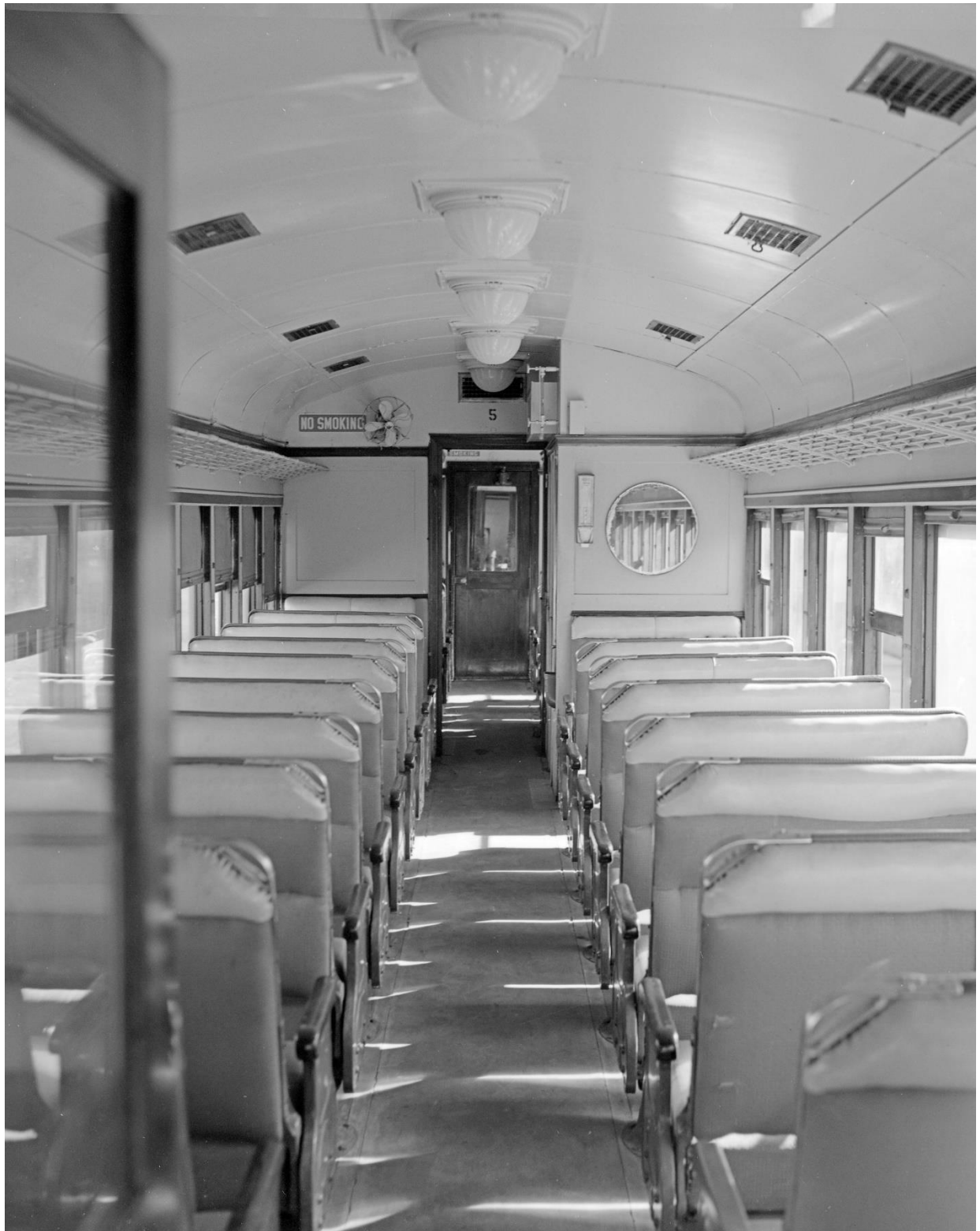
Inside car #5 the interior woodwork was painted, an electric water cooler was installed, and a mirror added. The limited modifications made to car #5 did not diminish the experience of riding an interurban, even in 1982 when this photograph was taken.
