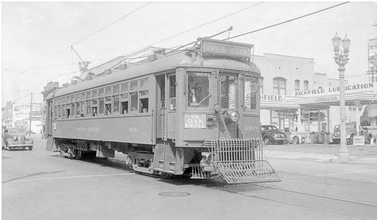
Steel roofs prevailed across all classes of steam railroad equipment including the interurban and suburban cars of the Southern Pacific. Pacific Electric car #1108, 31 August 1941. (Photographer credit: Victor Vincent DuBrutz).
