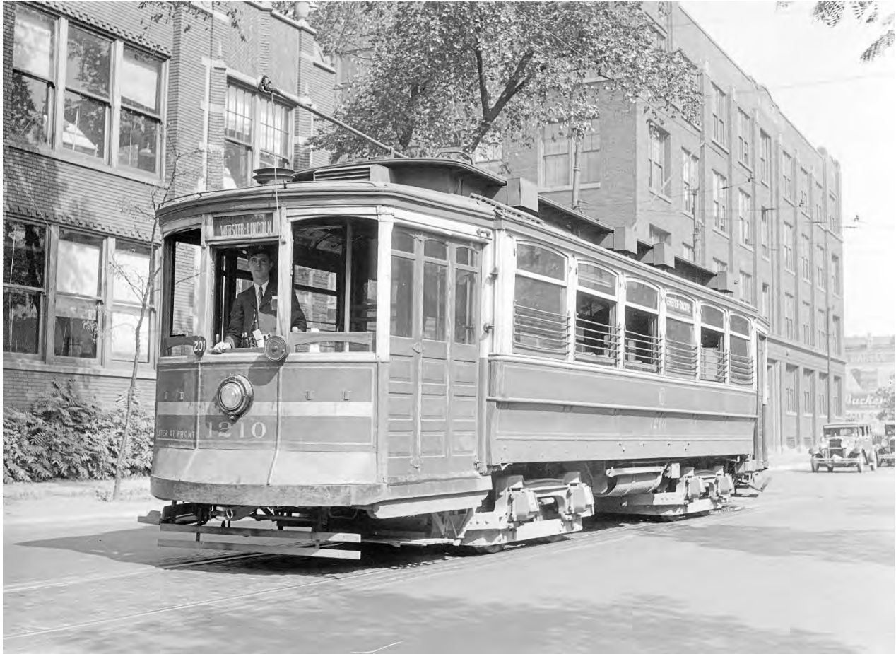
Chicago Surface Lines car #1210 at Racine and Fullerton, circa 1930. The architecture of this car was typical of small streetcars built at the end of the 19th and the beginning of the 20th centuries. These cars are distinguishable from interurbans of the same era by their wide loading platforms, single compartments, and deck roofs with a free-standing clerestory.
