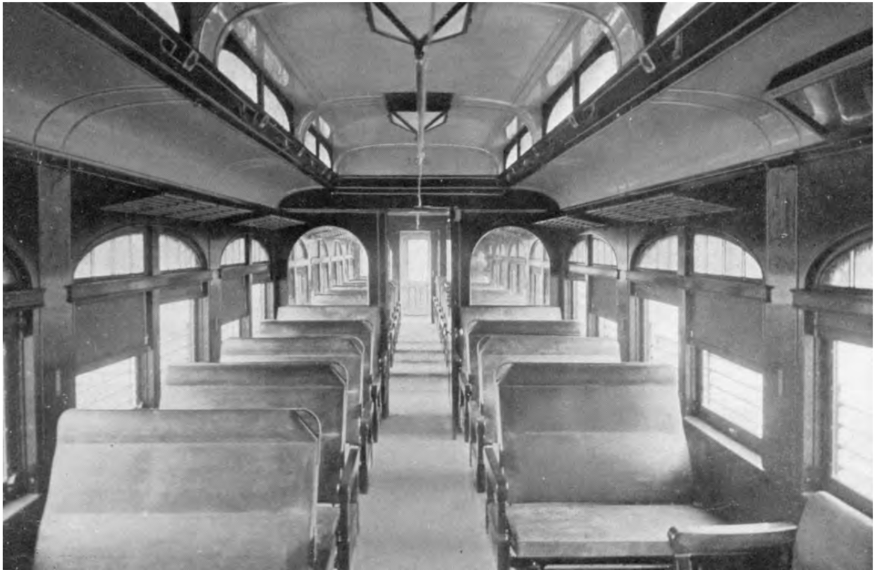
The Chicago, Lake Shore and South Bend Railway (South Shore Lines) coach trailer car #108 at the G.C. Kuhlman Car Co., Cleveland, O., 1908. 53 The South Shore Lines cars were a cut above the ordinary at the start: typical interurban cars of the era used bare bulb light fixtures and walkover seats without extra padding at both the bottom and top of the back. The extra padding gave better back and neck support than the seats normally provided by street railways or some steam railroads.
