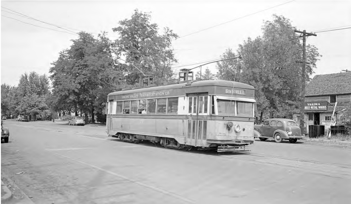
J.G. Brill Company built small standardized “Master Unit” cars for both street railways and interurbans. The weight per square foot of floor area was 106.8 lbs. This car was built for Yakima Valley Transit in 1930. 6th Street, Yakima, Washington, 19 August 1946.
