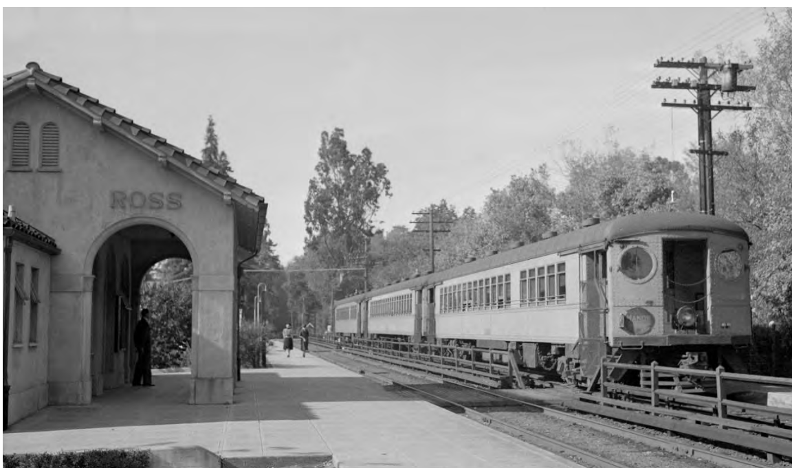
A modified version of the SP East Bay cars was built in 1929 for the suburban services in Marin County operated by SP subsidiary Northwestern Pacific (NWP). The NWP cars offered more leg room and could seat only 103 passengers but included nifty amenities such as heat that were originally lacking on the East Bay cars. Ross, Marin County, California, 1940. (Photographer credit for two images: Victor Vincent DuBrutz).
