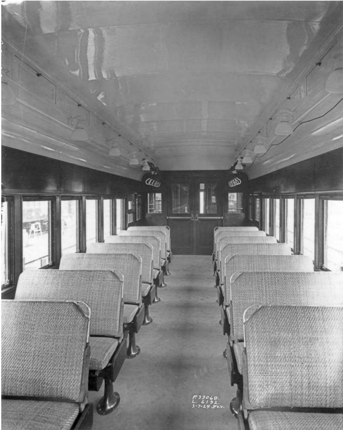
Illinois Central electric self-propelled suburban commuter car, Pullman, 7 March 1929. In its austerity, gone from the Baltimore and Ohio railroad day coach above are decorative ceiling stripes, overhead center lamps, fans, baggage racks, arm rests, and mohair upholstery. Instead, there is an assumption that the majority of passengers on crowded rush period trains will not get a seat on their journey home. This car seated 84 but was expected to accommodate 109 standees. Just inside the vestibule doors, there are porcelain-coated straps for standees to hold on to while the train lurched from station to station. (Photographer credit: John P. Van Vorst for Pullman Car & Manufacturing Company).
