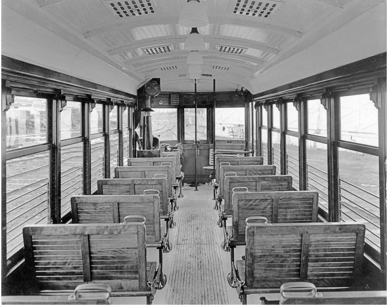
Wood slat seats in an uninsulated interior was less than attractive in its day. Revived Birney operations at Fort Collins, Colorado, and Fort Smith, Arkansas, have proved popular with tourists and have endured, nonetheless. This car was built for Detroit, Michigan, but is typical of Birney interiors.
