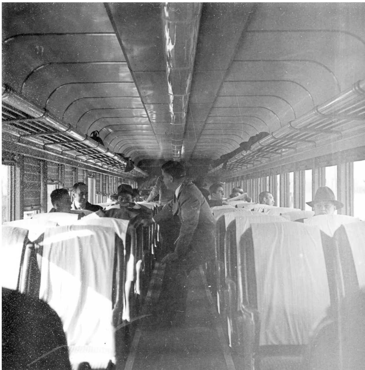
Car #203 was unique among the stretched trailers. It was modernized with fluorescent lighting and forced-air ventilation; the other five stretched trailers retained their incandescent center lamps and roof mounted vents.
