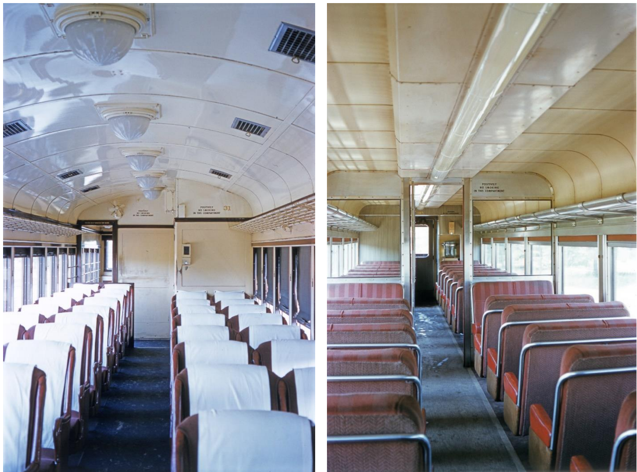
Typical car before (left) and after lengthening and air-conditioning (right). The lowered ceiling carried the ventilation system and fluorescent lighting. The new aluminum baggage racks were easier to reach and held larger parcels. The new foam rubber seats rotated on a turntable base as had the original seats so that passengers faced forward with the direction of travel. The interiors of the air-conditioned cars were arranged with a compartment for smoking separated by a swinging door, while the sealed picture windows reduced the levels of outside dirt and noise.
