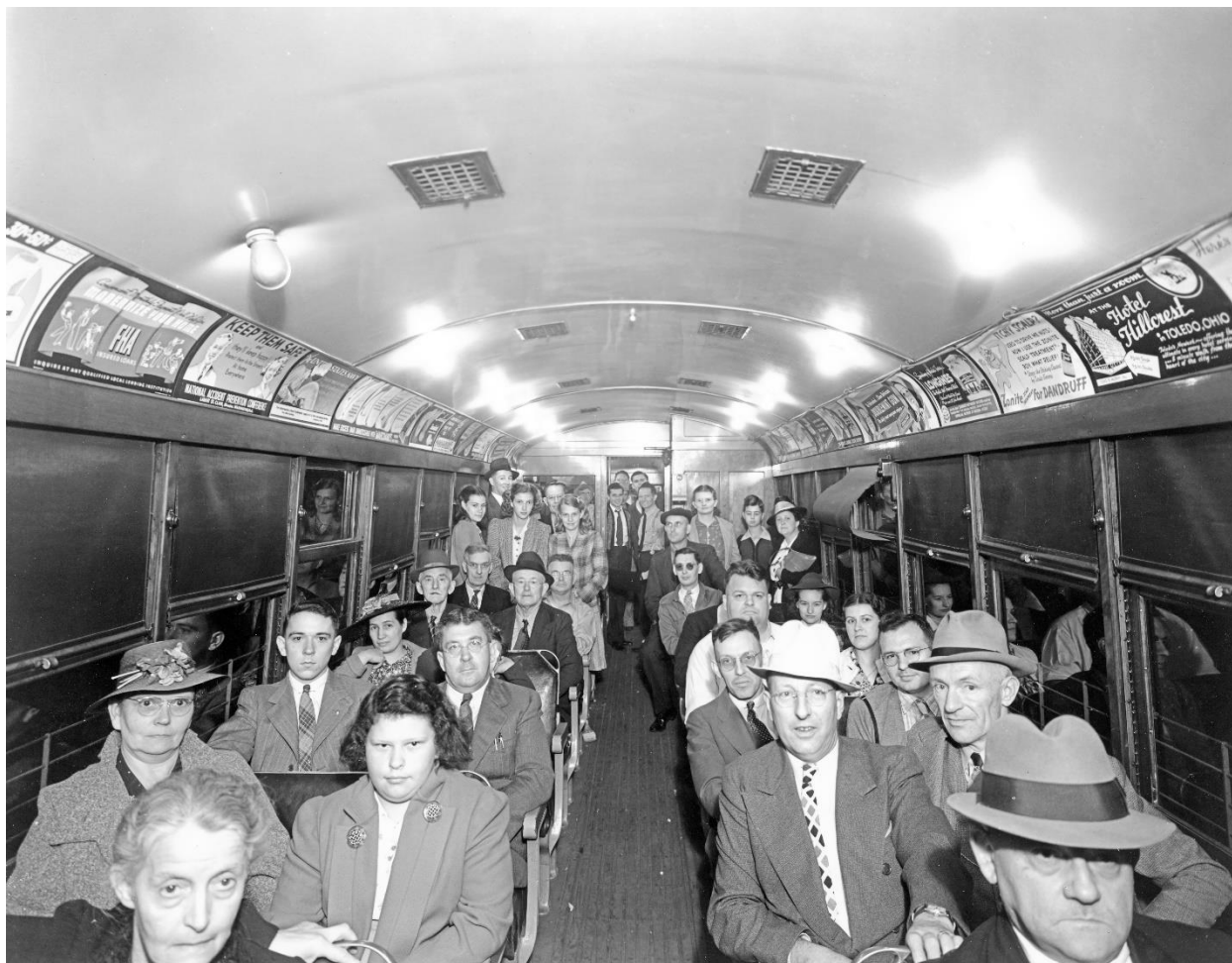
Stark Electric curved-side lightweight car #42, 16 July 1939. Lightweight coaches were divided into main and smoking compartments in the same manner as heavyweight cars. The toilet is on the right side of the image ahead of the partition. Car #42 was built in 1926, was 46' 3" long, and could seat 52. This large crowd had turned out for the last run of the Canton to Salem, Ohio, interurban. (Photographer credit: Dimit Brothers Photographers, Alliance, Ohio).
