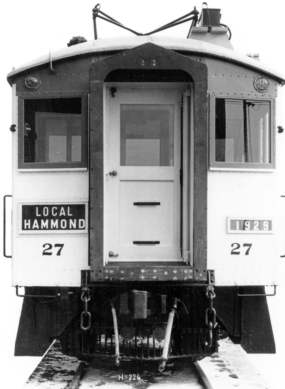
South Shore Line car #27, Standard Steel Car Company, Hammond, Indiana, 1929. The diaphragms and buffers were manufactured by the Waugh Draft Gear Company of Chicago. A standard Adams & Westlake diaphragm curtain meant to keep fingers away from the steel plates while the train is in motion is mounted to the right (non-cab) body collision post. (Photographer credit: Standard Steel Car Company).
