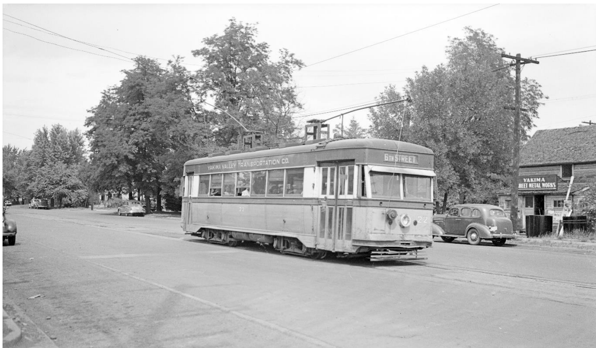
J.G. Brill Company built small standardized “Master Unit” cars for both street railways and interurbans. The weight per square foot of floor area was 106.8 lbs. This car was built for Yakima Valley Transit in 1930. 6th Street, Yakima, Washington, 19 August 1946. (Photographer credit: Victor Vinzent DuBrutz).
