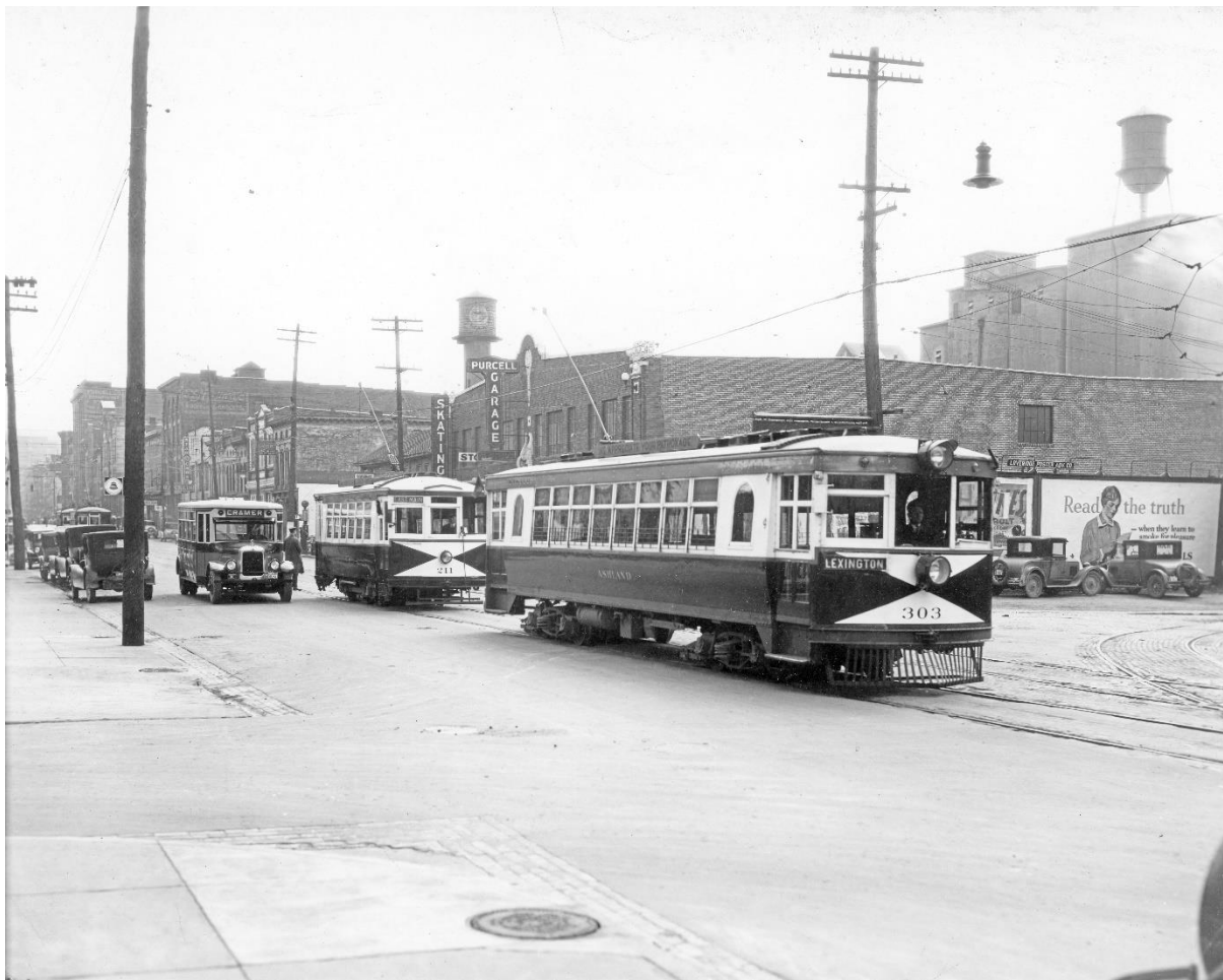
Kentucky Traction & Terminal Cincinnati Curved-Side interurban coach at Lexington, 1928. These small cars were among the lightest interurban cars built on the basis of weight per passenger. Per Kentucky Jim Crow statutes, these small cars had separate “colored” seating compartments. (Photographer credit: Lafayette Studio, Lexington; R.J. Lang, proprietor).
