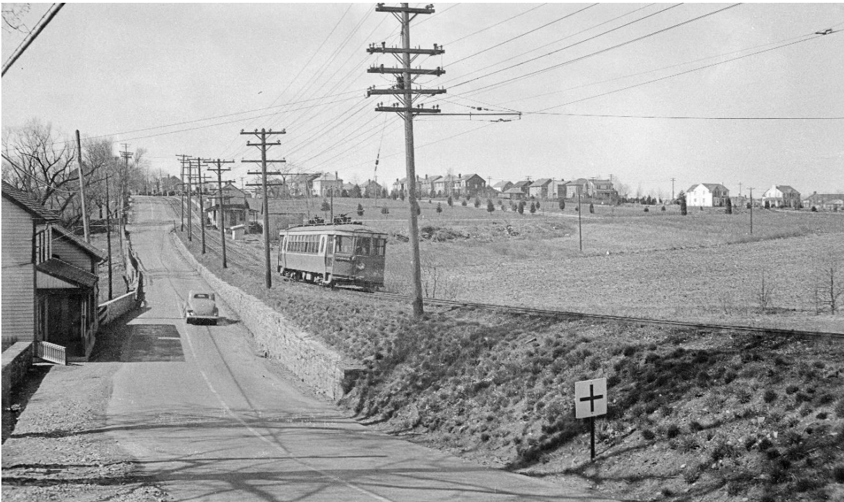
Lightweight curved-side cars were nearly exclusively used on lines with declining traffic and deteriorating track typical of much of the interurban network in the mid-1920s. This car operated on the Conestoga Traction Company near Ephrata, Pennsylvania.
