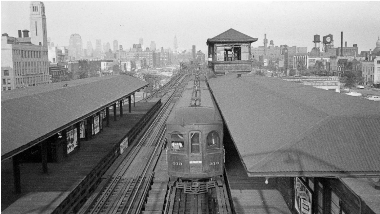
Sunset Lines car #313, Marshfield Avenue, Chicago, 21 August 1953. Interurban cars that operated over Chicago's 'L' were constrained by everything seen and unseen in this view. The pedestrian bridge that served as the photographer's perch limited the height of these cars.
