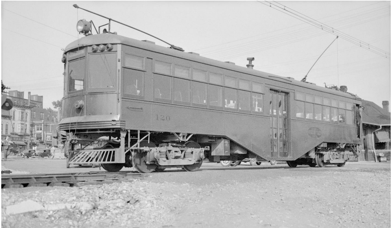
Center-entrance car of the East St. Louis & Suburban, Alton, Illinois, 9 September 1934. This was one of four identical cars built in the company shops in 1924. The Alton, Granite & St. Louis bought five nearly identical cars in 1917 from American Car Company.
