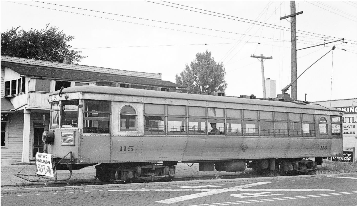
Curved-Side lightweight car on the Toledo & Indiana. Similar cars were purchased for street railways as these small cars were well suited to both city and interurban service.
