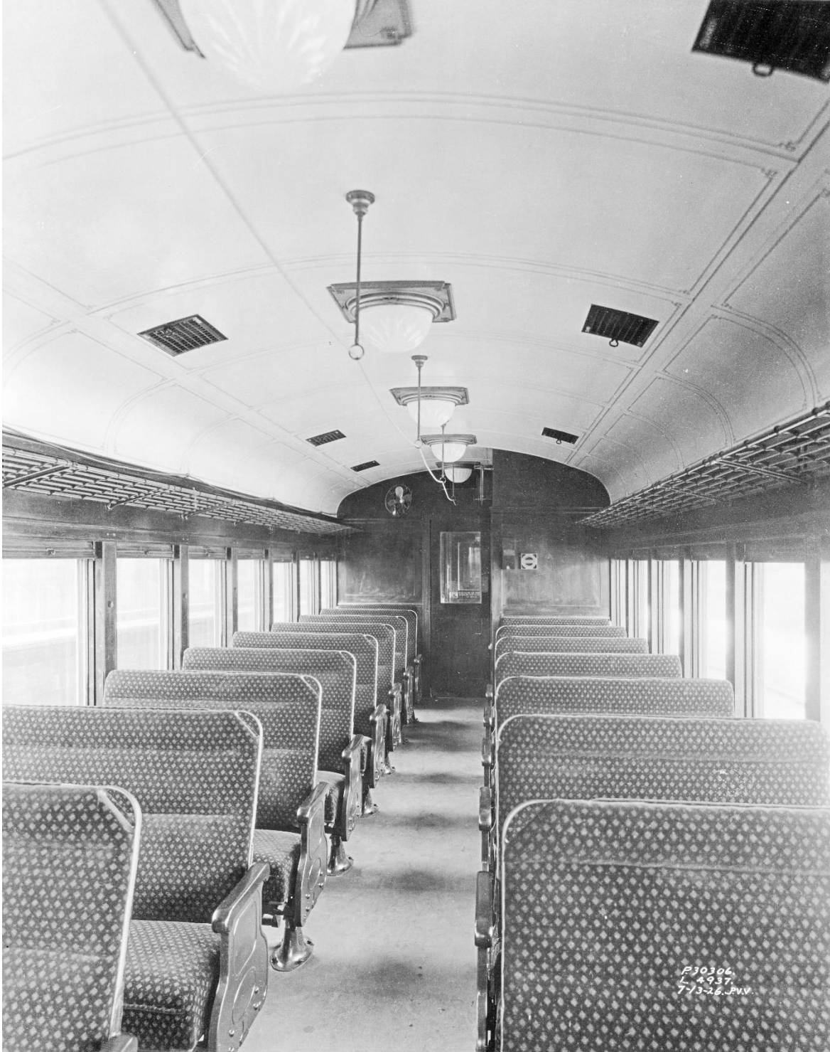
The short and happy evolution of the South Shore Line passenger car fleet: the first coaches were delivered in 1926. The smoking compartment was beyond the door at the center of the image. The seats in the main compartment were upholstered in green patterned "cut, no-cut" German mohair; the seats in the smoking compartment were imitation leather. Car #3 at Pullman, 13 July 1926. (Photographer credit: John P. Van Vorst for Pullman Car & Manufacturing Company).
