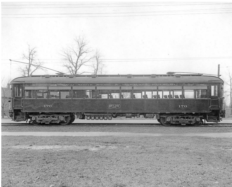
Chicago, North Shore and Milwaukee Railroad (CNS&M) car #170 at Highwood, Illinois, 1920. Floor and side-panel framing gives this car a light and airy interior, but a weak structure. Cars delivered to CNS&M in 1928 and 1930 used heavier truss-side framing.
