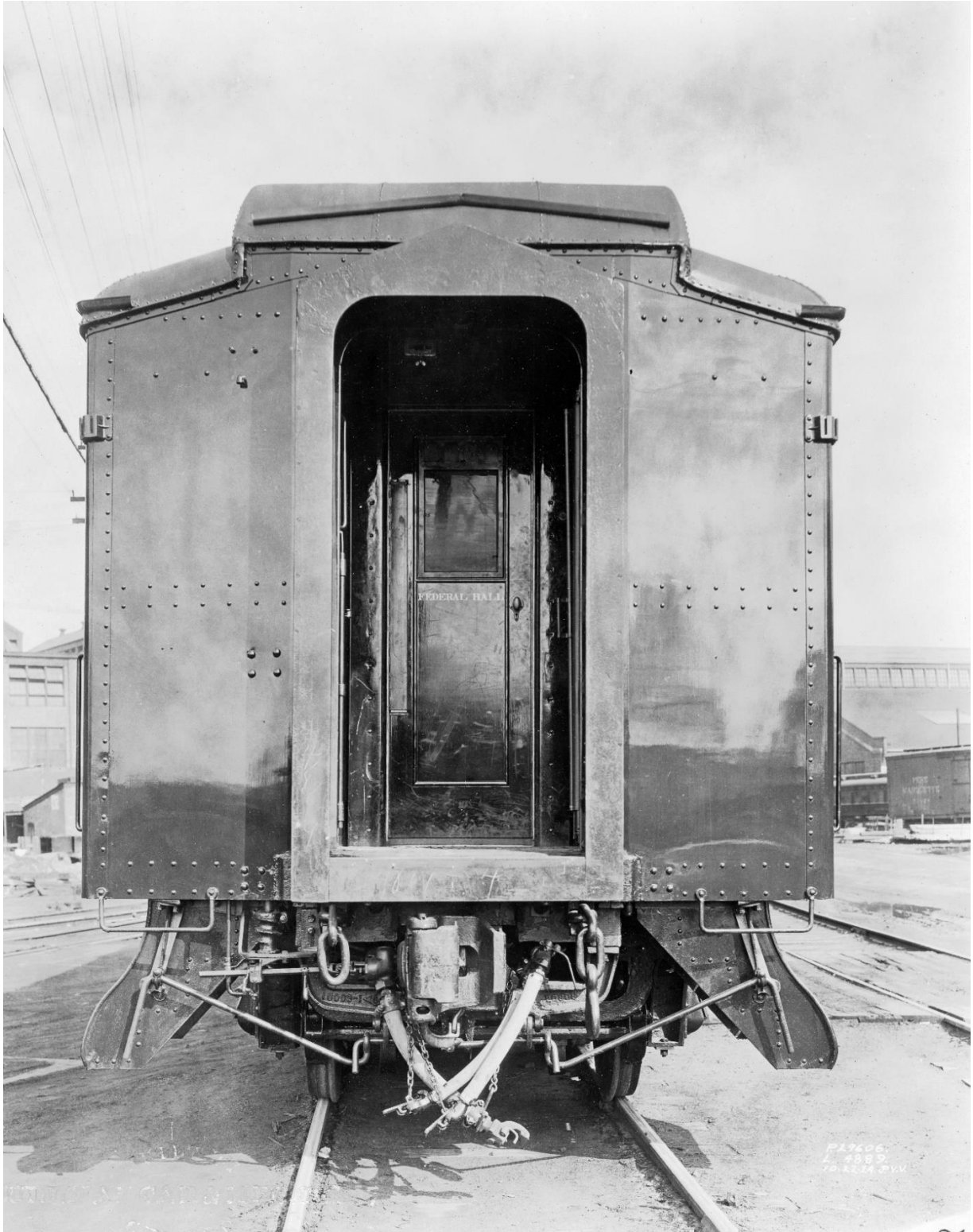
Pullman observation car Federal Hall at Pullman, 22 October 1924. The Waugh diaphragm at the end of Federal Hall is identical to those installed on the South Shore Line coaches and deluxe cars. (Photographer credit: John P. Van Vorst for Pullman Car & Manufacturing Co.)
