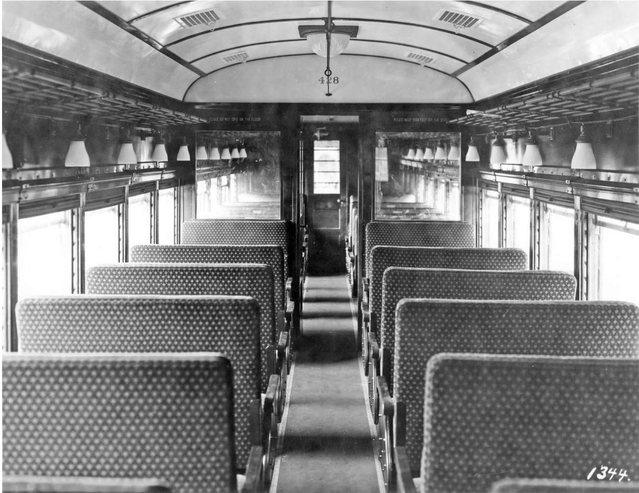
Indiana Union Traction car #428, combination coach-baggage car interior, view toward the front, St. Louis Car Company, November 1925. After the interurban carbuilders adopted steel for construction, the interior layout of the cars remained unchanged: there were still separate compartments for the general public, smokers, and baggage. This car was equipped to operate as a single unit, in multiple with other combination coach-baggage cars, or with a parlor-observation-buffet car on the Indianapolis-Fort Wayne runs. (Image Courtesy of the John W. Barriger III National Railroad Library).
