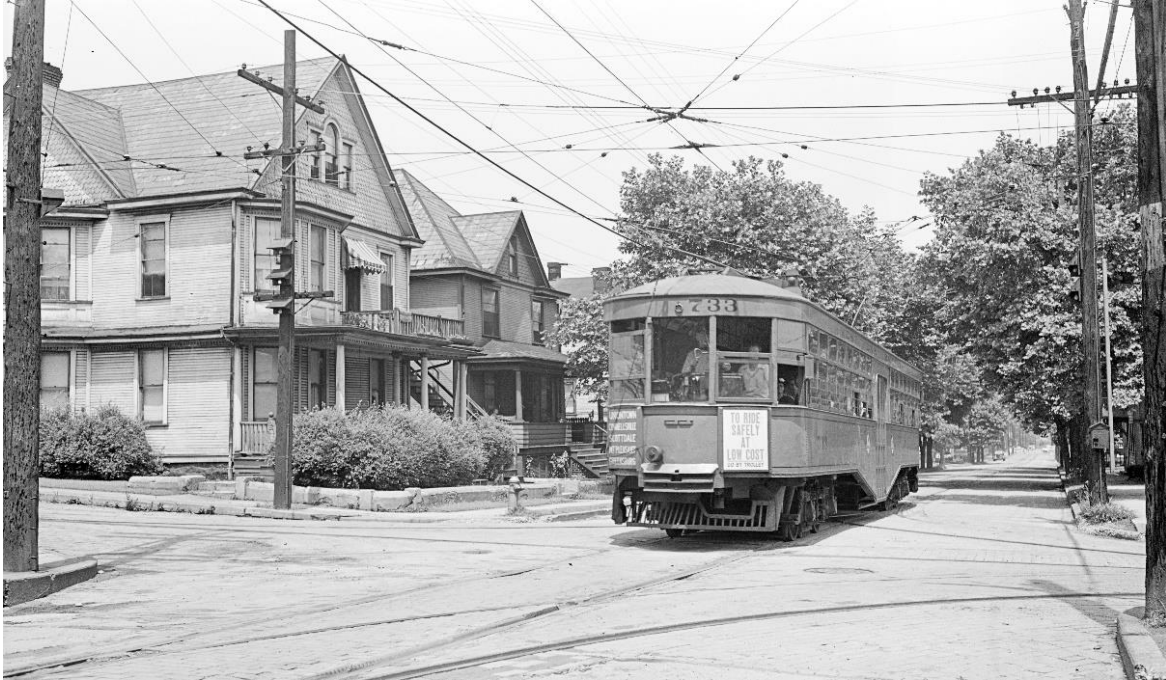
West Penn Railways built their own cars in the company shops at Connellsville. Car #733 was built in 1923, thirteen years after the first cars of this design were delivered by the Cincinnati Car Company. The weight of these cars per square foot of floor area was identical to the Yakima cars pictured above – 106.8 lbs. Connellsville, Pennsylvania, 4 July 1948.
