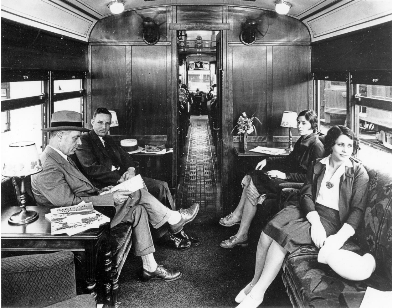
Cincinnati & Lake Erie Red Devil car #124. This single car constituted an entire train. The coach section is up front; parlor car customers were seated at the rear. (Photographer credit: Mayfield Photo Service, Dayton, Ohio).
