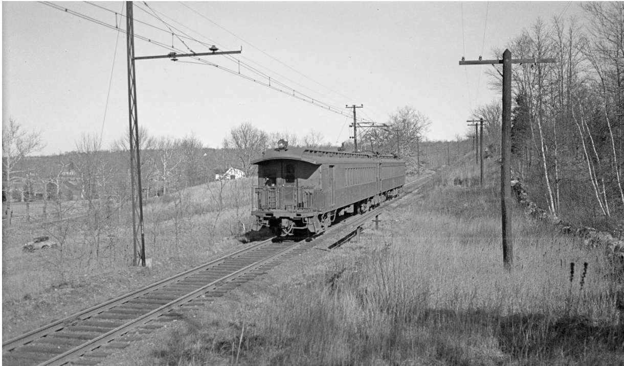
The New York, New Haven & Hartford line from New Canaan to Stamford was the first North American steam railroad electrification of a branch line for suburban service, completed in 1901. Electric suburban trains reached New York City on 24 July 1907. This train was bound for Stamford at Woodway, Connecticut, 11 November 1937.
