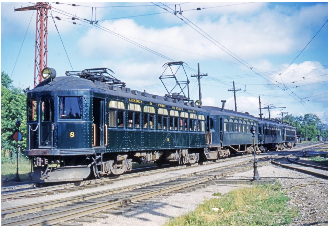
London & Port Stanley interurban car #8. The diagonal rivets above the bolsters and at the center of the car attach the side sheathing to the pressed-steel side-panel inner truss – a key feature of the Stillwell design. The active structure of the car continues up through the windows and across the steel roof with its ogee curves. The floor frame is only a secondary support. (Photographer credit: Wilbourne B. Cox).
