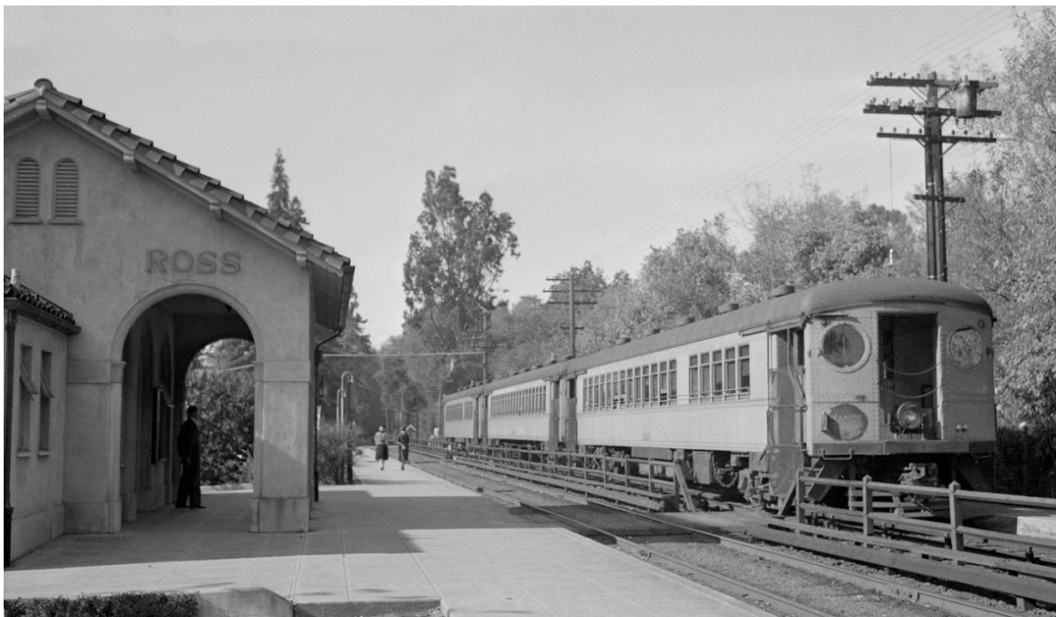
A modified version of the SP East Bay cars was built in 1929 for the suburban services in Marin County operated by SP subsidiary Northwestern Pacific (NWP). The NWP cars offered more leg room and could seat only 103 passengers but included nifty amenities such as heat that were originally lacking on the East Bay cars. Ross, Marin County, California, 1940. (Photographer credit for two images: Victor Vinzent DuBrutz).
