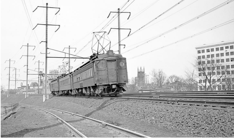
The largest fleet of electric commuter cars in the United States were the 1,428 MP-54 cars of the Pennsylvania Railroad and its subsidiary companies, Long Island Railroad and Pennsylvania-Reading Seashore Lines. Construction of cars of this design spanned 30 years – from 1908 through 1937. The last MP54s had yet to be delivered when this photo was taken at Elizabeth, New Jersey, 29 March 1936.
