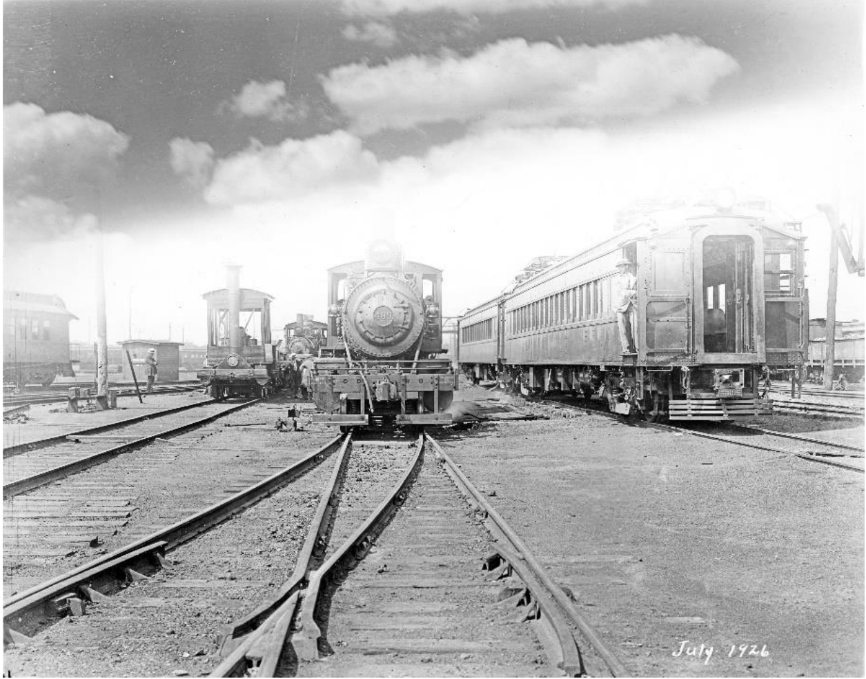
The first cars of the general design of the DL&W equipment were built by Pullman for the Illinois Central suburban service in 1921 for operation from Chicago to the South Side and South Suburbs. The first of these cars were initially hauled by steam locomotives while planning for the electrification was underway. Chicago, Illinois, July 1926.
