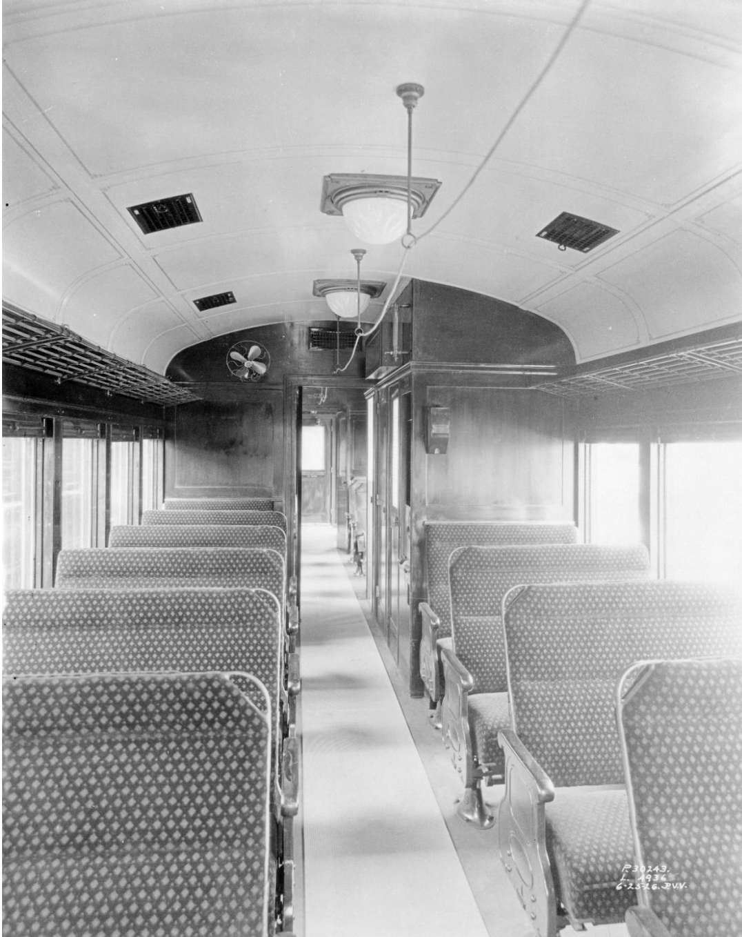
Combination coach-baggage car #106, at Pullman, 25 June 1926. This view is from the back of the main compartment looking toward the front of the car. Beyond the first partition is the smoking compartment, and past the second is the baggage room. This arrangement is identical to that of CSB&NI combination coach-baggage car #305, supra.
