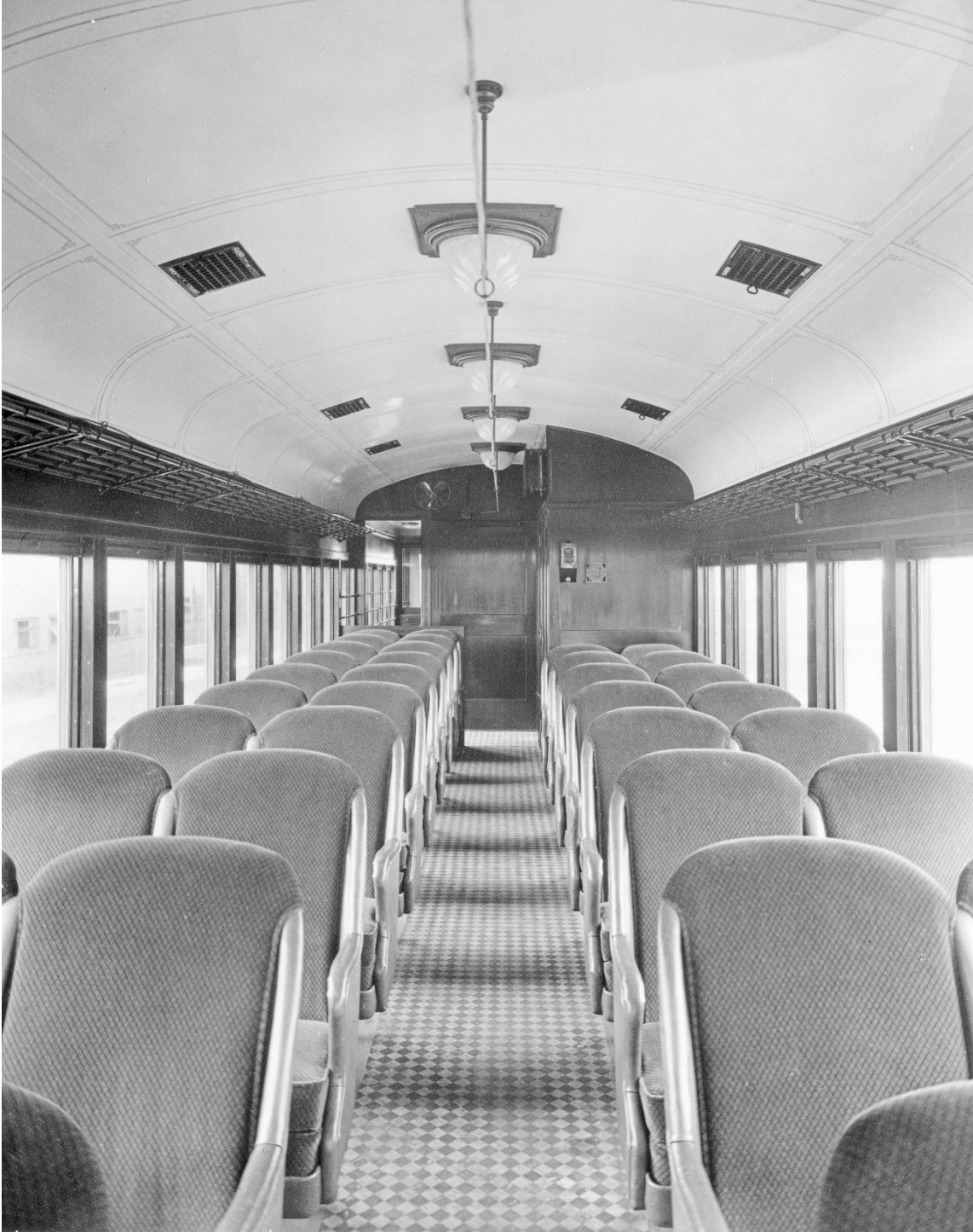
South Shore Line car #27 at Standard Steel Car Company, Hammond, Indiana, circa February 1929. This was the final form of the South Shore Line coaches. The improvements in the car interiors between the final two car orders were insignificant: the aisle partition between the main and smoking compartments was eliminated, patterned linoleum graced the floor, and seating manufacturer Hale & Kilburn had increased the arch of the seat backs for a refined appearance. Other minor changes from the earlier cars included a different style of center lamp. (Photographer credit: Standard Steel Car Company).
