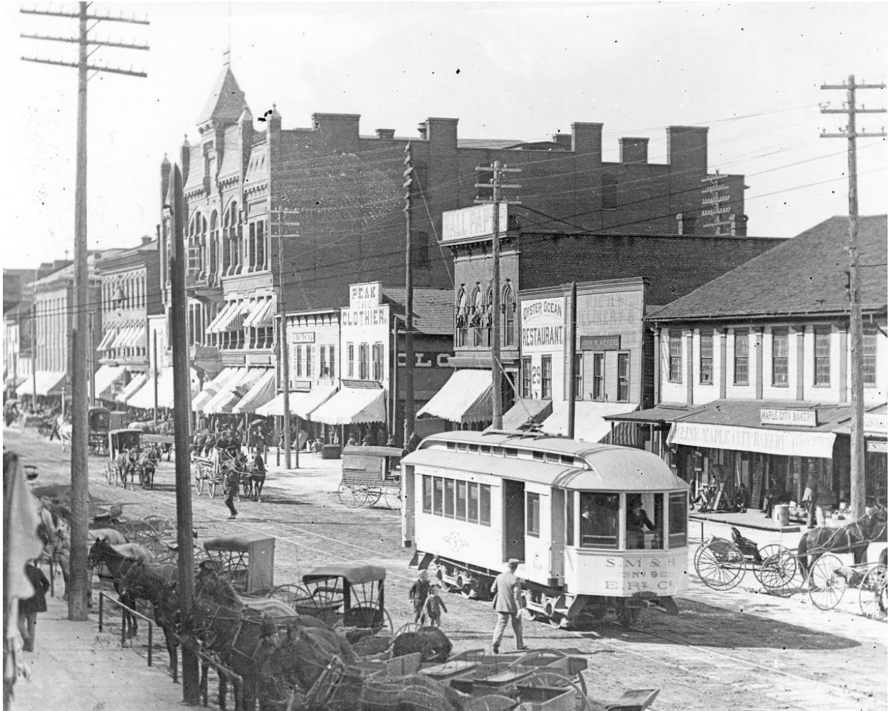
Pioneer Sandusky, Milan and Norwalk (SM&N) car #9 at Norwalk, Ohio, 1893. Although lettered for the Sandusky Milan and Huron, the corporate name had changed after the cars were lettered, but before they were delivered. These small cars were typical of the pioneer interurbans. The dimensions of SM&N car #9 are similar to the early streetcar pictured below.
