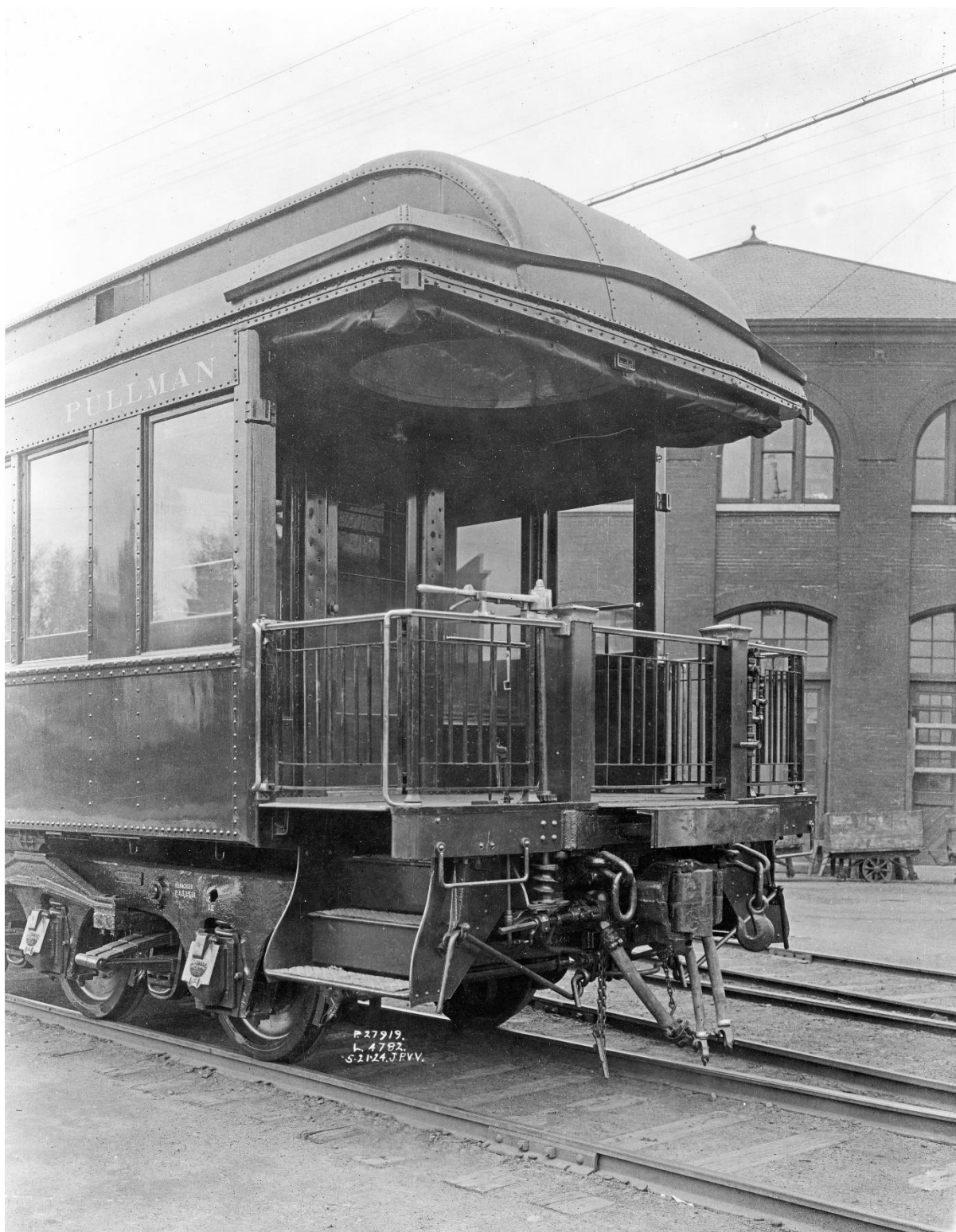
Pullman observation car Great Northern at Pullman, 21 May 1924. The trucks under the Great Northern are one-piece castings with 5" x 9" journals and with straight equalizers – a modern truck for their time built over two years before the trucks under the South Shore Line deluxe cars. (Photographer credit: John P. Van Vorst for Pullman Car & Manufacturing).
