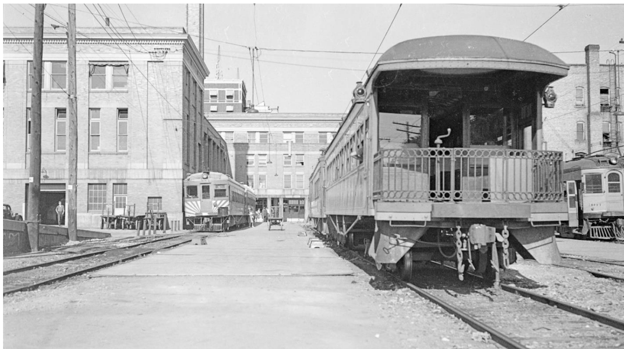
SL&U parlor-observation car at Salt Lake City, circa 1946. The builder, Niles Car & Manufacturing (Niles) primarily built wood interurbans and streetcars. This steel car constructed in 1916 was exceptionally light weight at 52,500 lbs. Niles did not survive long into the steel car era and was out of the carbuilding business in 1917. 31
