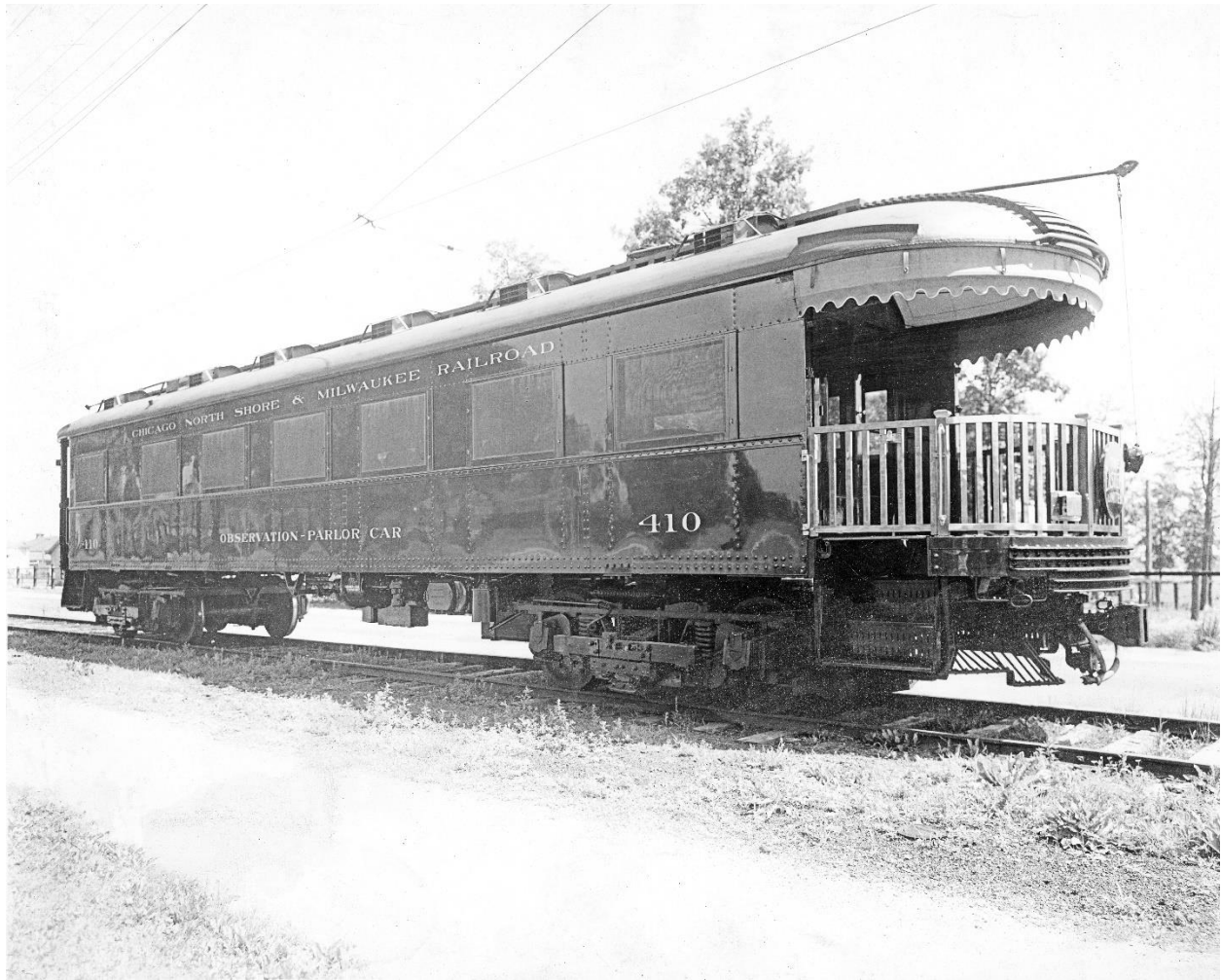
North Shore Line parlor-observation car #410, Highwood, Illinois, 1923. An air compressor was not often standard equipment on a non-motorized car, but car #410 has a compressor just ahead of the rear truck. Most often, non-motorized cars received their air supply from powered cars in the same way that a locomotive supplies air to all the cars in a passenger or freight train. Here, the air compressor has the effect of making this car heavier than it would be without this mechanical equipment, and makes it more difficult to compare the finished weight of the car with other cars of the same class of service including the South Shore Line parlor-observation cars. (Photographer credit: Commercial Department, Chicago, North Shore and Milwaukee Railroad).
