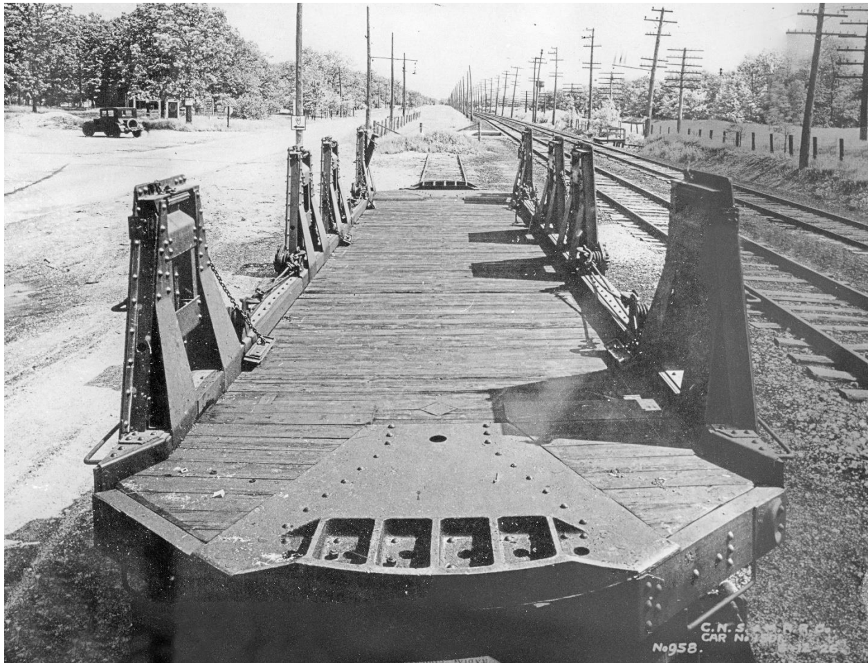
First-of-its-kind flat car for handling highway trailers, 12 June 1926. The car shown, #1501, had appliances typical of interurbans including tapered ends and radial couplers to negotiate sharp curves.
