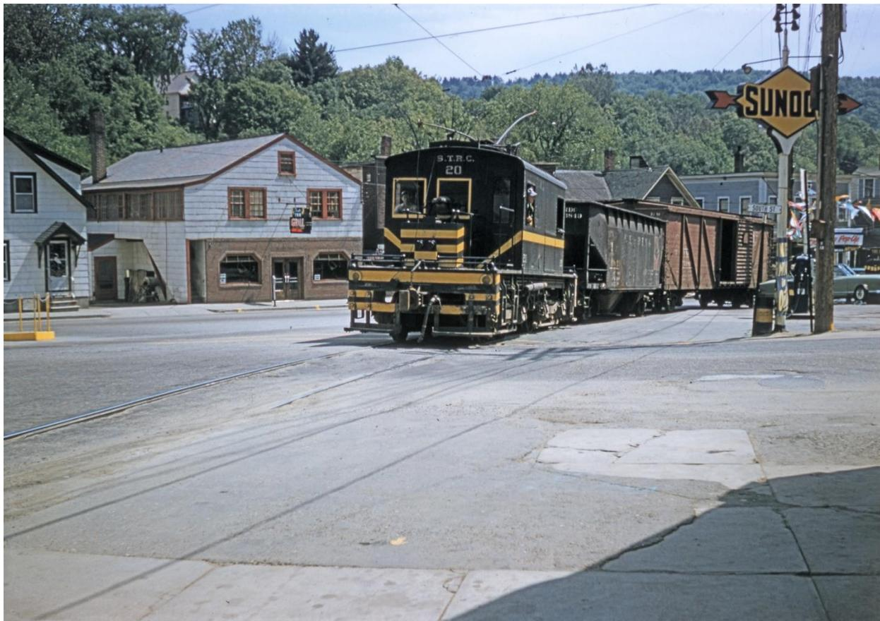
*Springfield Terminal Railway (ST) Baldwin Westinghouse locomotive #20 at Main and South streets, Springfield, Vermont, 20 June 1956. ST operations were hampered by steep grades, sharp curves, and street running, but it was the only rail access to the machine tool industries of Springfield, Vermont. The capital stock of ST was accumulated by the Boston & Maine Railroad in just over a decade beginning in 1922.*
